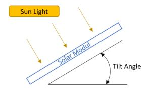
The solar modules must be set up at an angle of at least 10° to the ground. Building regulations must be observed.
