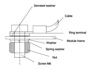
The solar modules are to be grounded according to the country-specific requirements and laws. If a lightning protection system is already present or intended to be installed on the building, the PV system is to be integrated into the protection concept against direct lightning strike. If a transformer less inverter is used, equipotential bonding may be prescribed in accordance with inverter manufacturer's specifications. Country-specific laws like NEC must observed.
